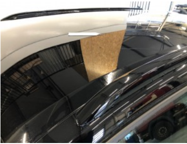
Roof - Restyle dent
