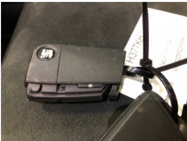
Sleutelbehuizing Reservesleutel Defect
