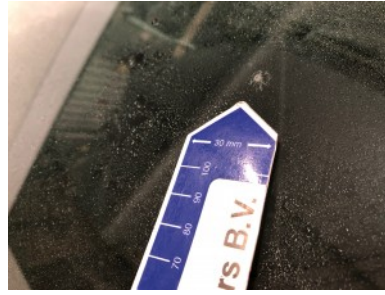
Windscreen - Stone chippings
