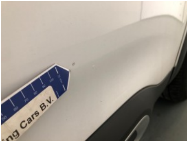
Front left door - Stone chippings
