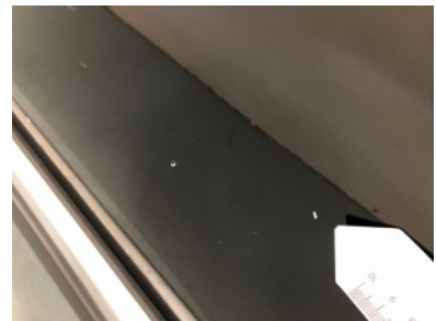
Front left door - Stone chippings
