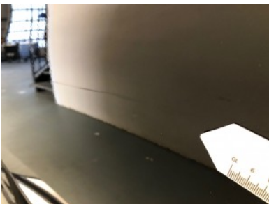
Rear right side window - Scratch
