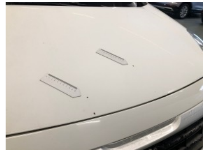
Grille - Stone chippings
