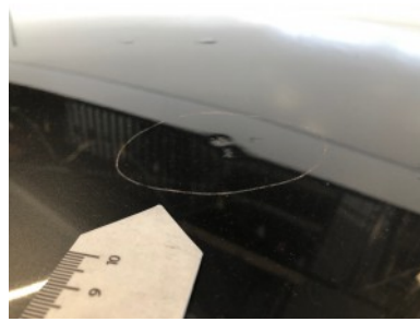
Roof - Restyle dent
