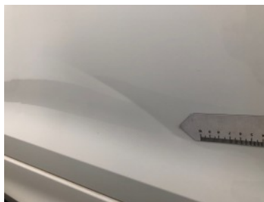
Rear right side window - Dent
