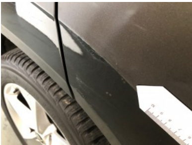
Rear right door - Paint repair
