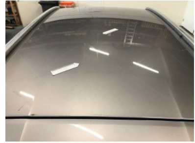
Roof - Hail damage
