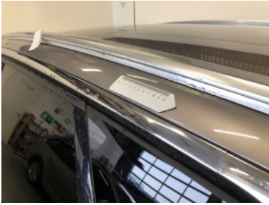
Roof - Hail damage
