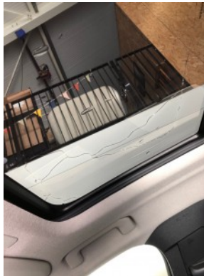
Roof - Hail damage
