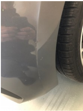
Rear bumper - Paint repair
