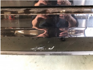
Rear bumper - Paint repair
