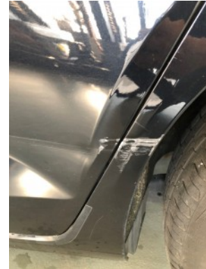
Rear left screen - Paint repair
