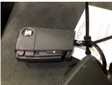
Sleutelbehuizing Reservesleutel Defect
